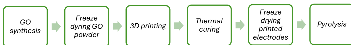
Figure 9. GO electrode manufacturing steps
