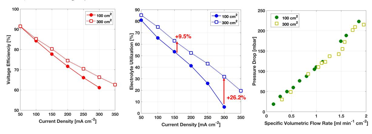
Considerable increase in voltage efficiency and electrolyte utilization due to the more even electrolyte distribution and no variation of pressure drops.
