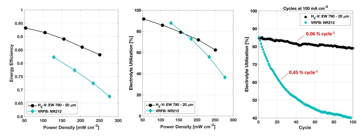
H<sub>2</sub>-V battery employing a thin membrane with reduced EW exceeds the performance of a VRFB with SoA components.
