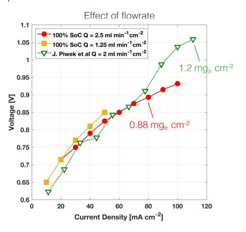
Both SoC and electrolyte flow rate affects V-O<sub>2</sub> performance, even at low operating current. At low operating temperature OER presents sluggish kinetic.
