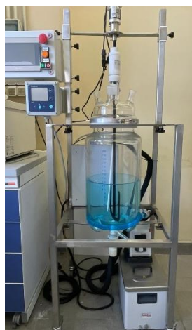
Fig. 5 25 L Reactor for scale up of the syntheses of NiMo heterogenous catalyst
