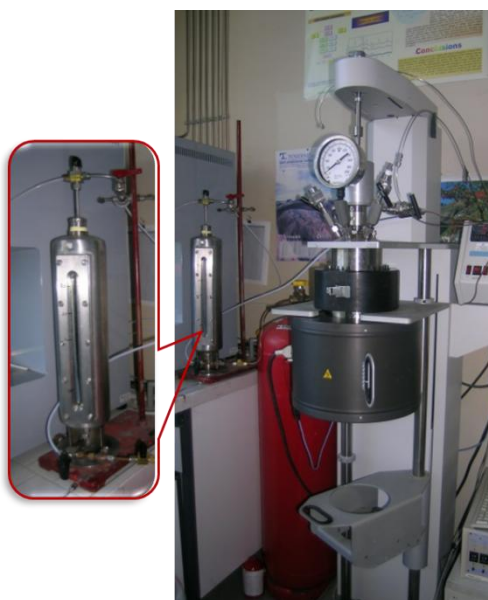
Fig. 1. Autoclave (2 L capacity) for the scale up of the syntheses of \text{MoS}_2/\text{C} heterogeneous catalyst
